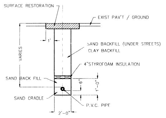
DETAIL OF SEWER PIPE INSTALLATION N.T.S.
