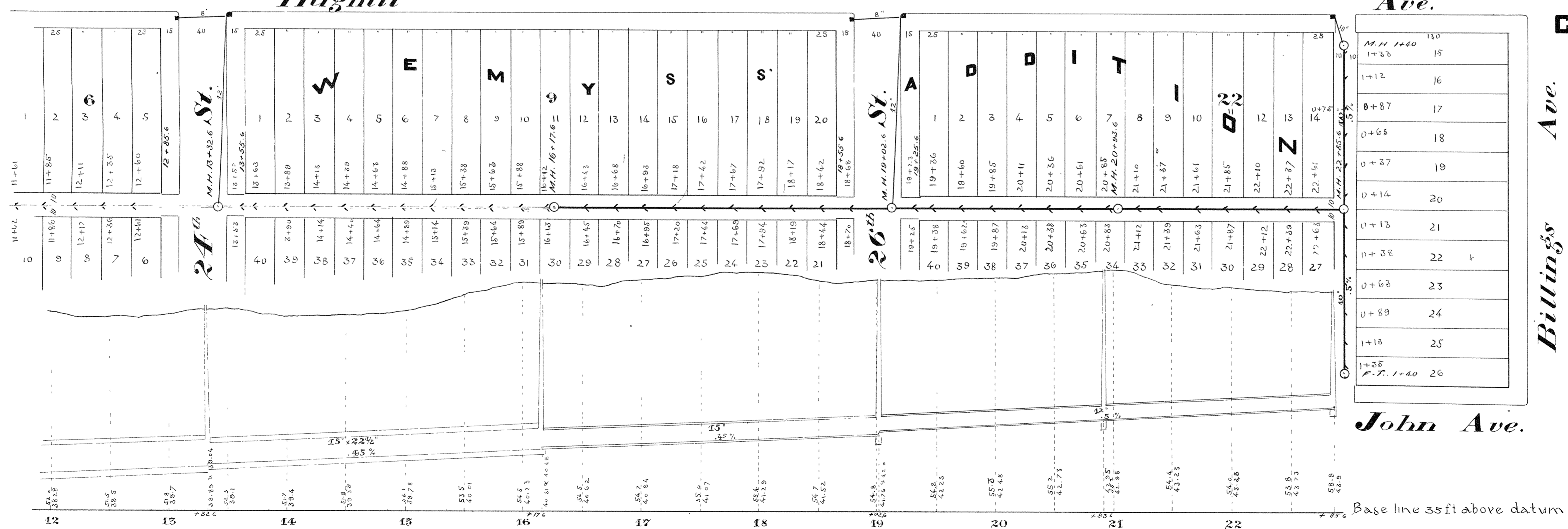
Plan & Profile of Sewer in Alley between John & Hughitt Aves. from Ritchie to Billings Ave.
