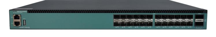
The E530 provides 440Gbps I/O bandwidth and 400G core bandwidth, combining a feature-rich switch core and an embedded ARM A53 CPU Core running at 800MHz/1.2GHz. The chipset supports a variety of port configurations, such as QSGMII and USXGMII-M, providing full-rate port capability from 100M to 100G in multiple configurations.
