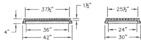
INLET CASTING TYPE "BP" CASTINGS SHALL BE NEENAH R-1878-B7G OR EQUAL WITH GRATE NOT TO SCALE
