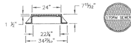
CASTING DETAIL TYPE "SL" CASTINGS SHALL BE NEENAH R-1670-A OR EQUAL, WITH TYPE "B" LID LETTERED "STORM SEWER", MACHINED BEARING SURFACES, ONE OPEN PICKHOLE NOT TO SCALE
