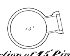
Section of 15" Pipe
