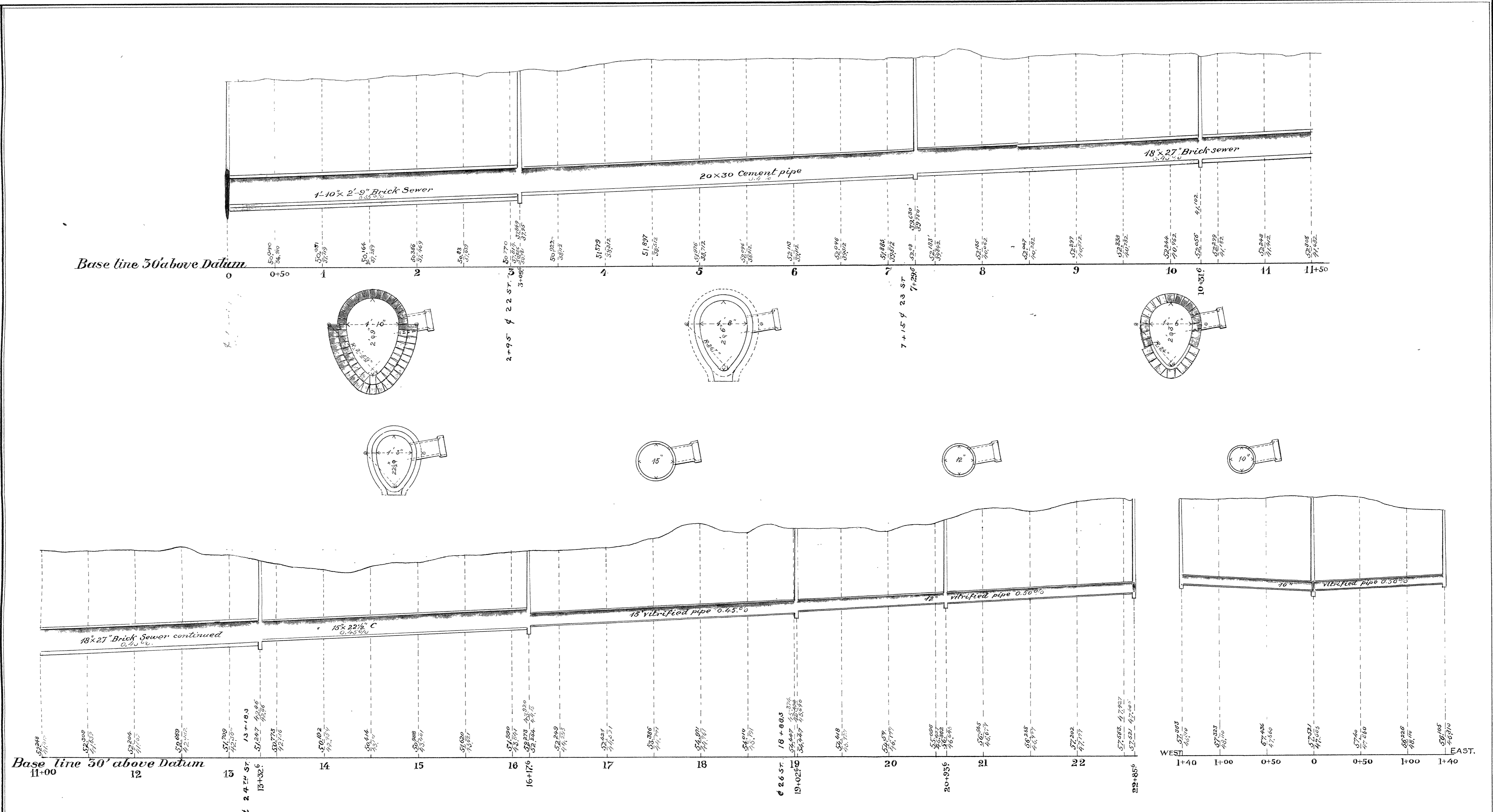
Profile of Sewer in Alley betw. Tower & Banks ave's from Alley S. of 21 st St. to Alley N of 28 th St. with E & W Laterals
