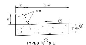
**CONCRETE CURB AND GUTTER 30"**
