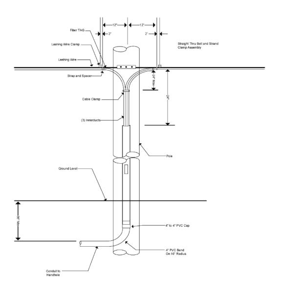
ALL RISERS INSTALLED ON CITY OF SUPERIOR JOINT OWNED POLES TO BE 4 INCH DIAMETER
