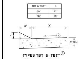
**CONCRETE CURB AND GUTTER**
