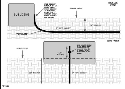
1. COORDINATION WITH THE PROJECT MANAGER SHOULD BE MADE BEFORE CONDUIT IS RAN TO ANY FACILITY. EXTERIOR BUILDING CONDUIT, HANDHOLES/PULL BOXES/VAULTS, CORE DRILLS, AND FIBER PULL LENGTH ARE DEPENDENT ON EACH FACILITY.
