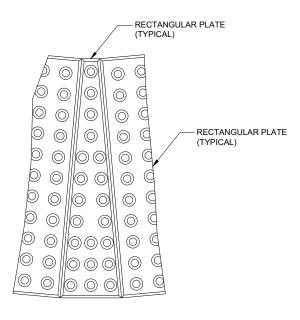
**PLAN VIEW RADIAL WEDGE PLATE CONNECTION DETAIL**
