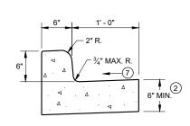
TYPES A D CONCRETE CURB AND GUTTER 18"
