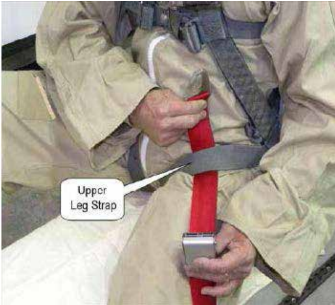
FIGURE 4. PASS TETHER LOOP UNDER UPPER LEG STRAP
