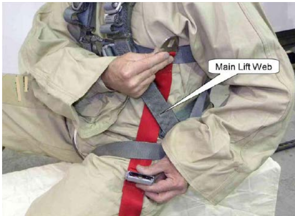
FIGURE 5. PASS TETHER LOOP UNDER MAIN LIFT WEB
