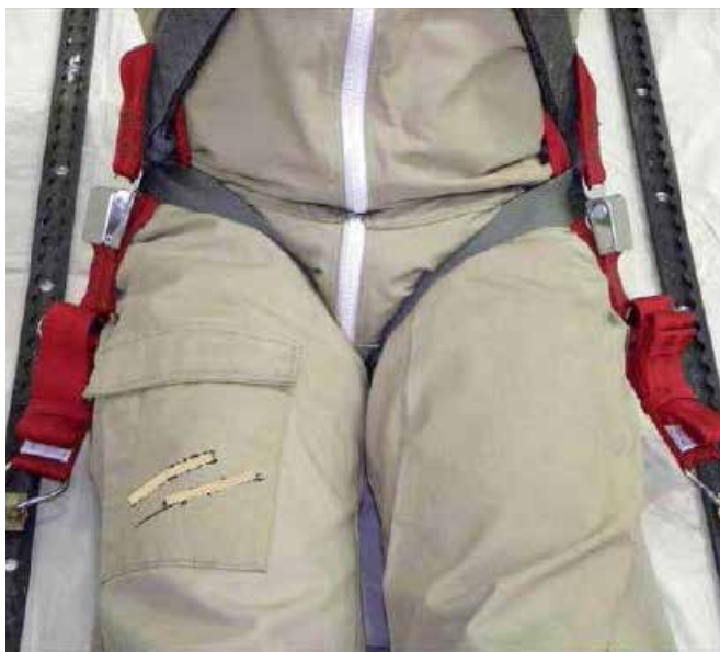
FIGURE 8. DUAL POINT, DUAL TETHER RESTRAINT CONFIGURATION FOR REAR-FACING FLOOR SEATS
