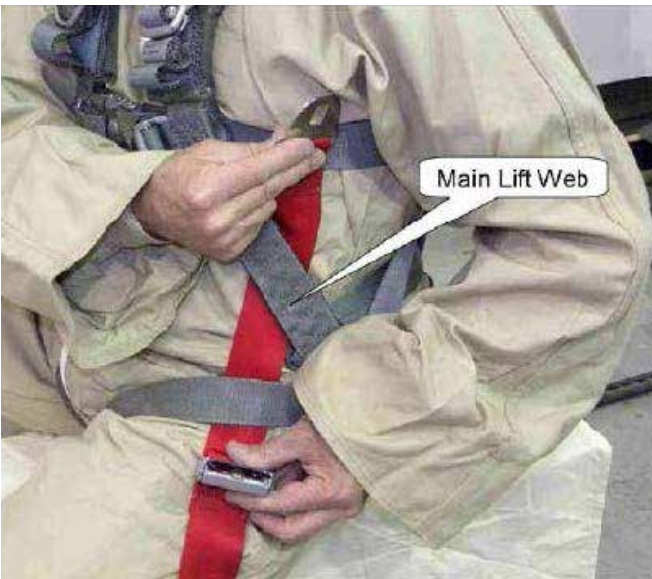
FIGURE 5. PASS TETHER LOOP UNDER MAIN LIFT WEB
