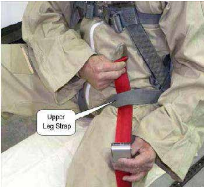
FIGURE 4. PASS TETHER LOOP UNDER UPPER LEG STRAP
